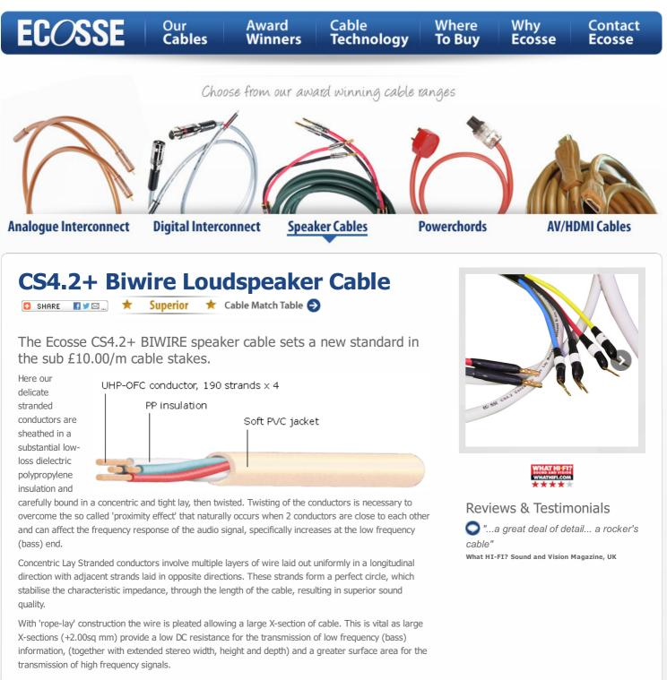
A loudspeaker consists of two drive units. - a high-frequency (HF) unit (tweeter), and a low frequency (LF) unit (woofer) they employ a "cross-over network" to direct low signal frequencies to the woofer, and high frequencies to the tweeter. This set up enables the loudspeaker to be bi-wired. In a biwire configuration 2 pairs of speaker cables are employed in order to ensure that the signals for
